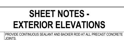
ALL INSIDE AND OUTSIDE CORNERS OF PRECAST TRIM TO NOT BE MITERED. EXTERIOR SIGNAGE ON BUILDING TO BE COORDINATED AND VERIFIED WITH ARCHITECT, OWNER AND SIGNAGE VENDOR. ALL VERTICAL INSIDE CORNERS TO HAVE 1/2" MOVEMENT JOINT.
