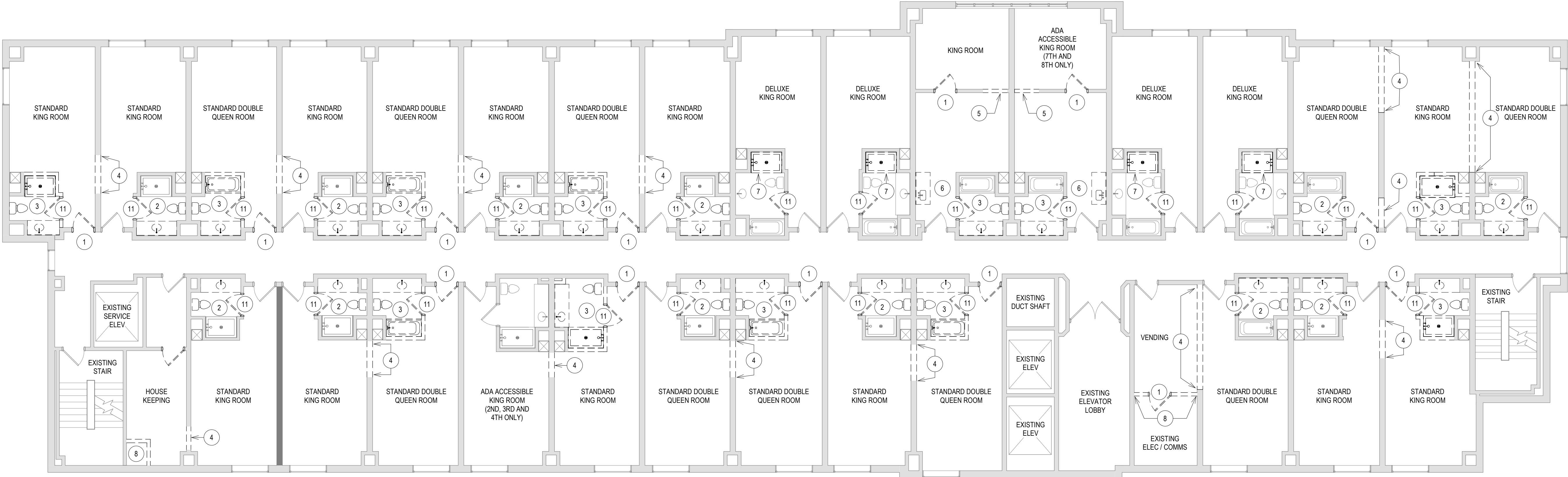
TYPICAL DEMOLITION PLAN - FLOOR 02-07 SCALE 1/8" = 1'-0"
