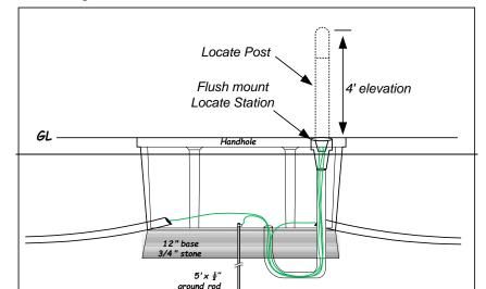
Detail Drawing of Handhole and Locate Station Installation
