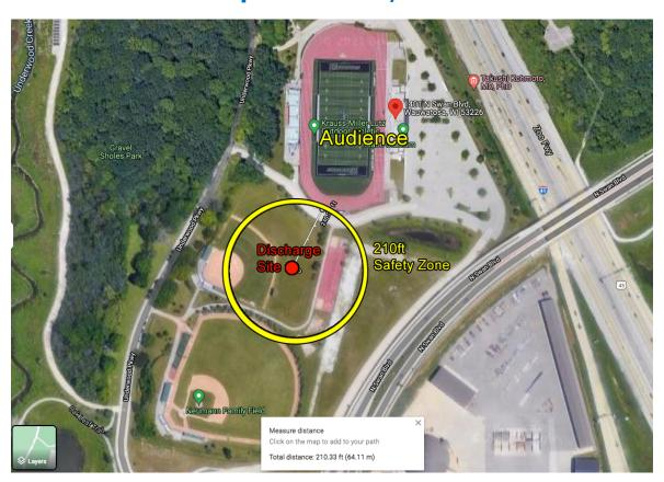
Discharge Site is in the ball diamond south of the football field. Up to 3" material will be used, requiring 210 feet of safety distance per NFPA 1123. The safety zone does not include the football stadium or track, and does not impinge on any roadways.
