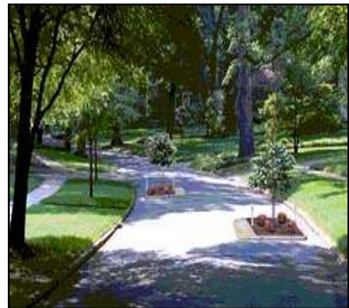
Example of chicane Resource: ITE Procedures and Warrants
