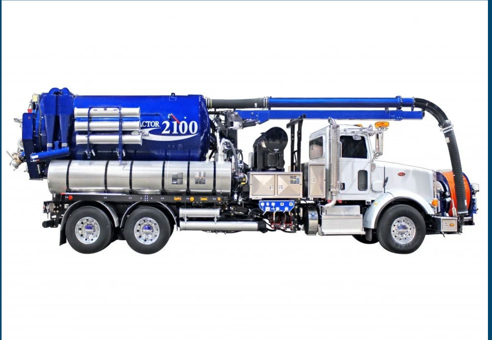
Vactor 2100i PD, 16" Vacuum, 15-yard Debris, Combo, 1500 Gallons Water
