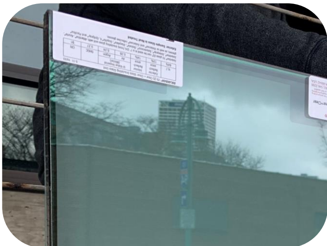
SPANDREL TO MATCH SOLARBAN 70 + OPACI-COAT
