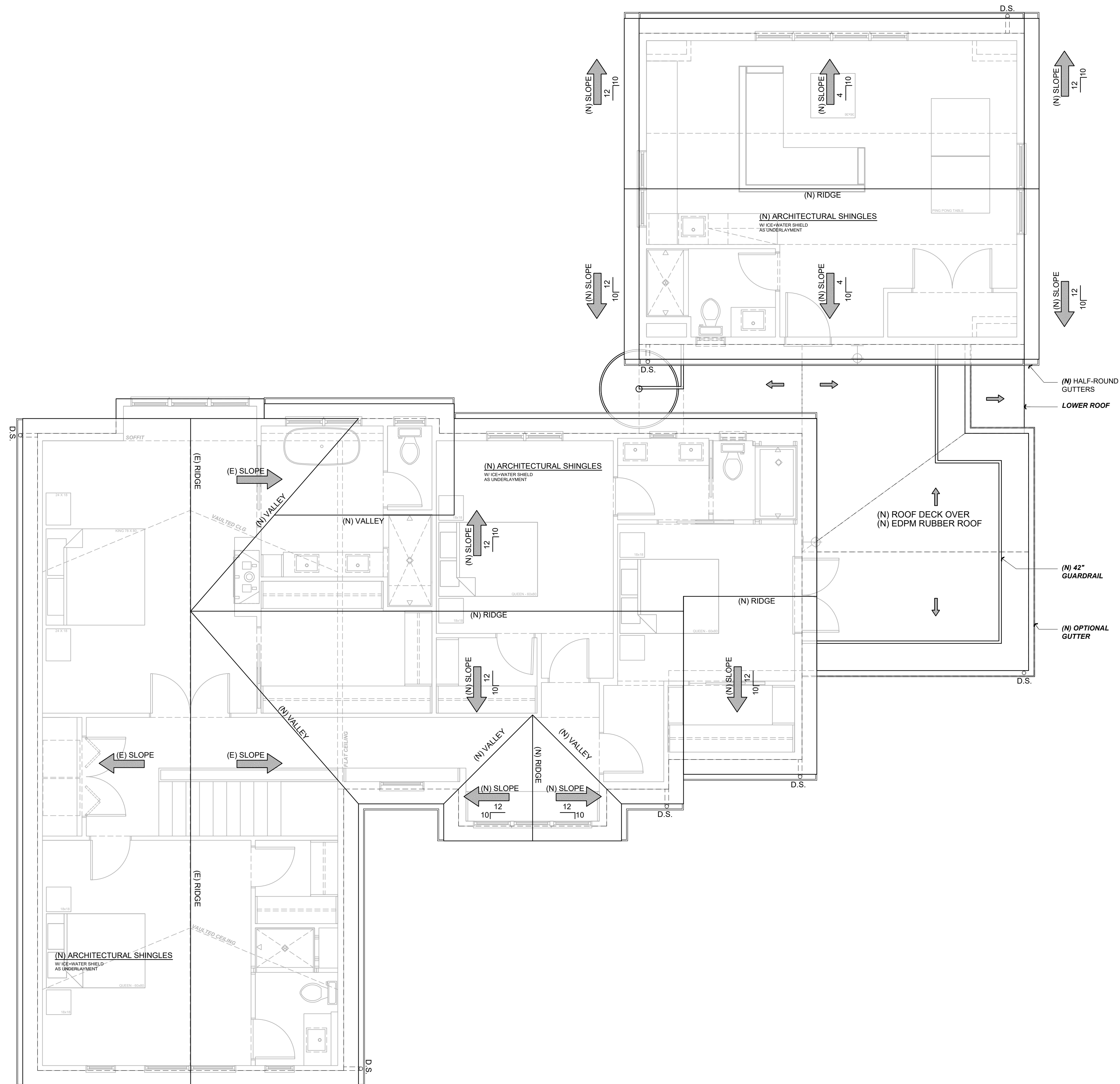
EXISTING/ PROPOSED ROOF PLAN Scale: 1/4" = 1'-0" 1 A2.2
