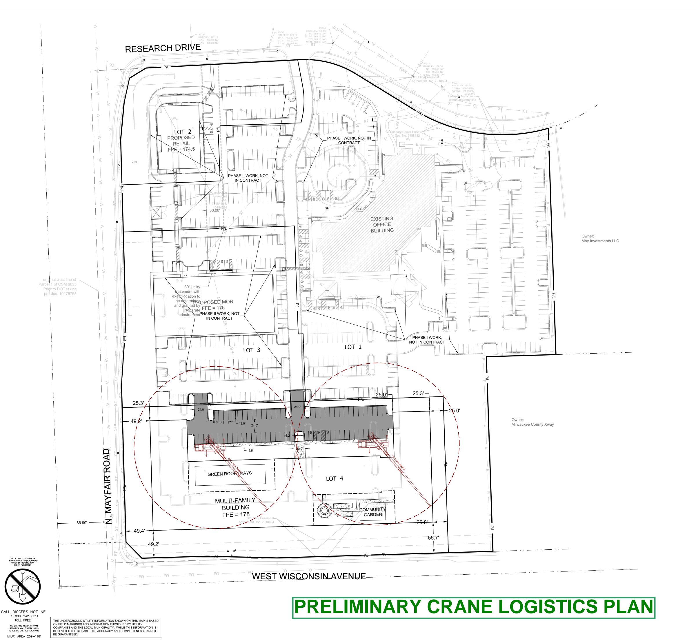
SITE INFORMATION SITE AREA 159746 3.667 AC SITE DISTURBED AREA 159746 3.667 AC 73350 1.684 AC 45.9 % EXISTING IMPERVIOUS AREA PROPOSED IMPERVIOUS AREA 95270 2.187 AC 59.6 % TOTAL PARKING SPACES 68 ADA PARKING SPACES 3
