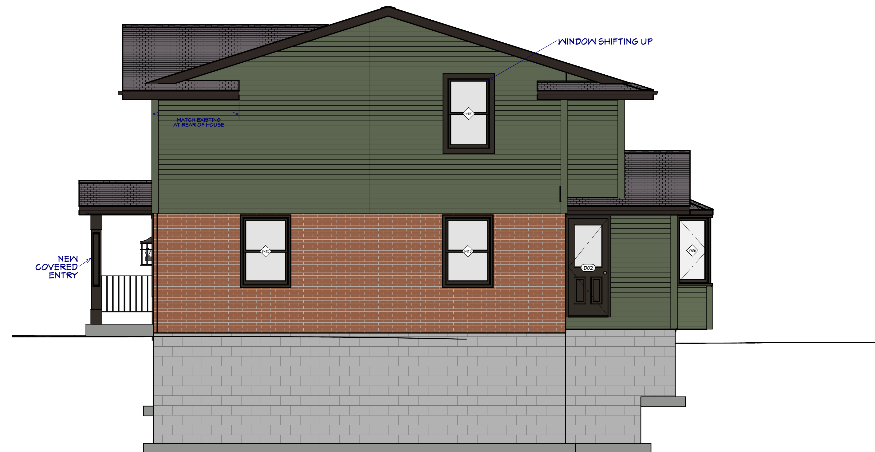
PROPOSED NORTH SIDE ELEVATION #4 1/4" = 1'-0"
